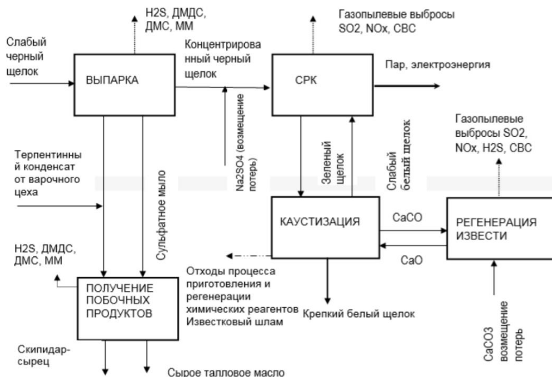
Figure 2.7 A block scheme showing the chemicals recovery process
