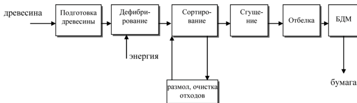
Figure 2.14 The stone-groundwood production process
